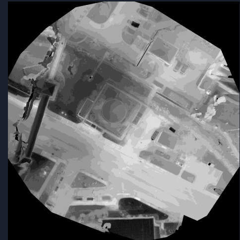
Figure 7. Thermal map of boiler building
