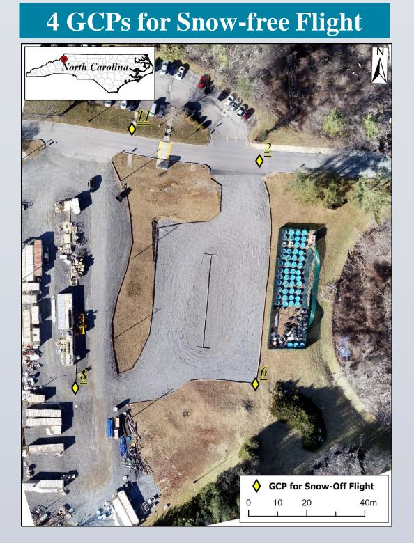
**<u>GCPs</u>**: handheld low-accuracy GPS Survey Strategy: the same 15 GCPs were used for the two drone flights
